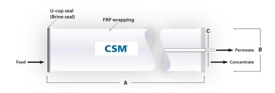
1. Each membrane element supplied with one brine seal, one interconnector (coupler) and four o-rings. 2. All RE8040 elements fit nominal 8.0 inch (203.2 mm) I.D. pressure vessels.
