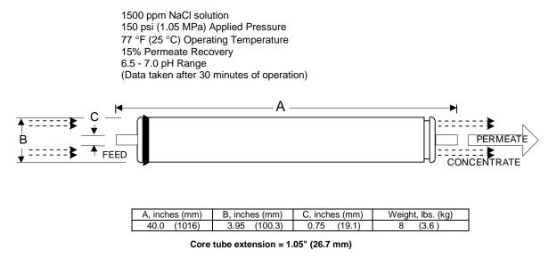
Notice: Permeate flow for individual elements may vary + or - 15 percent. All membrane elements are supplied with a brine seal, interconnector, and o-rings. Elements are enclosed in a sealed polyethylene bag containing less than 1% sodium meta-bisulfite solution and then packaged in a cardboard box.
