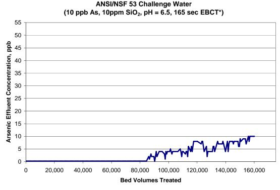
Figure 3. ADSORBSIA™ As500 media dynamic arsenic adsorption at pH 6.5, with low arsenic level. \*EBCT = empty bed contact time
