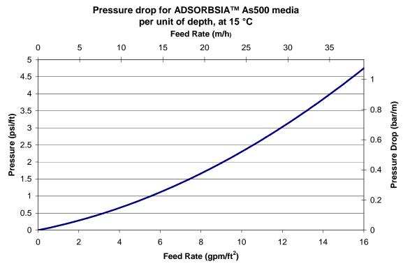
Figure 5. Pressure drop as a function of feed rate.
